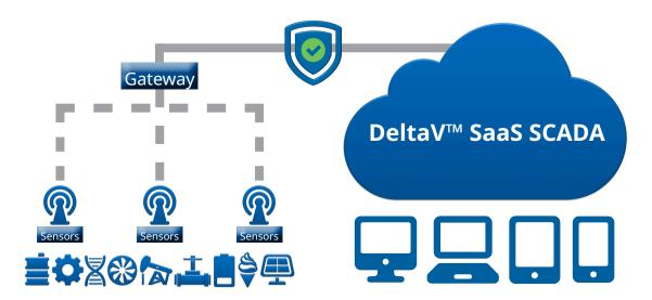
We simplify the connection between sensors to get you the data you need to make better business decisions. Emerson's DeltaV™ SaaS SCADA provides both a web interface to end users, as well as the ability to push data to third party platforms giving you accurate operation data, remote control, cry-out alarms and the mobility you need to increase your production, profits and sustainability.
